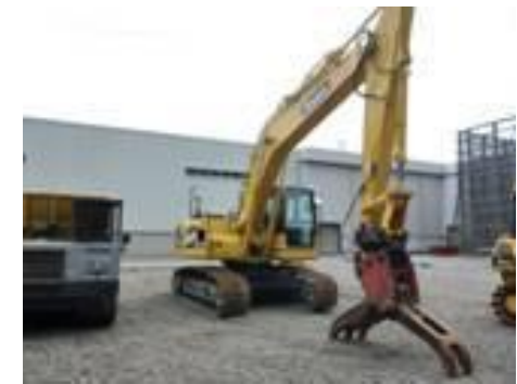
Hydraulic shovel (Tip of the arm is replaceable)
